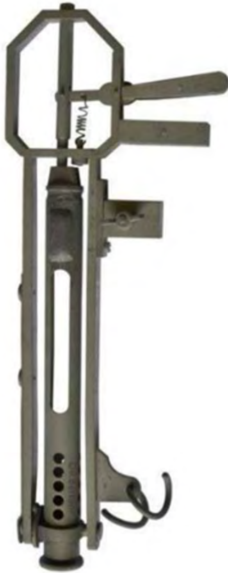
Messenger operated mounting for reversing thermometer (Negretti & Zambra, Londra, UK). 1910-1920.
