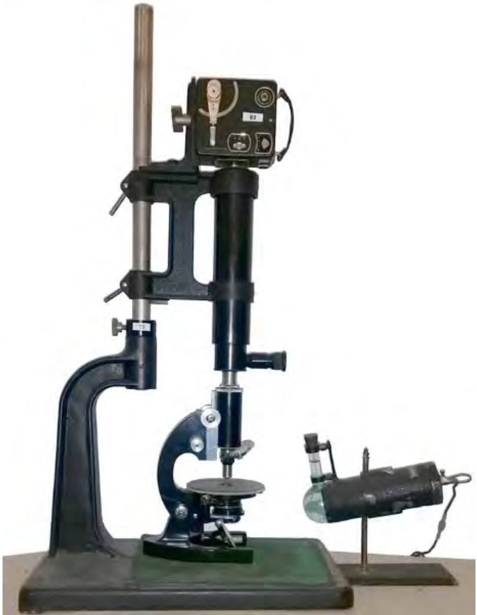
Baldi's microcinematography system. End of the 1930s
