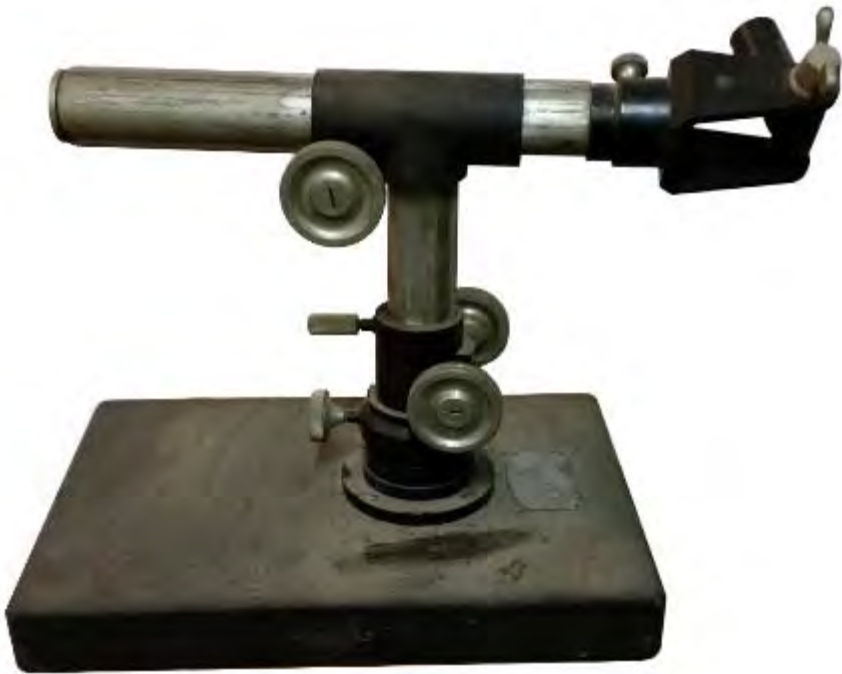
Articulating arm for binocular microscope.
