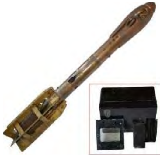
Batitermograph Thermarine (Wallace & Tieman, New Jersey, USA).1950. Right box: coated glass slides and graph reader.
