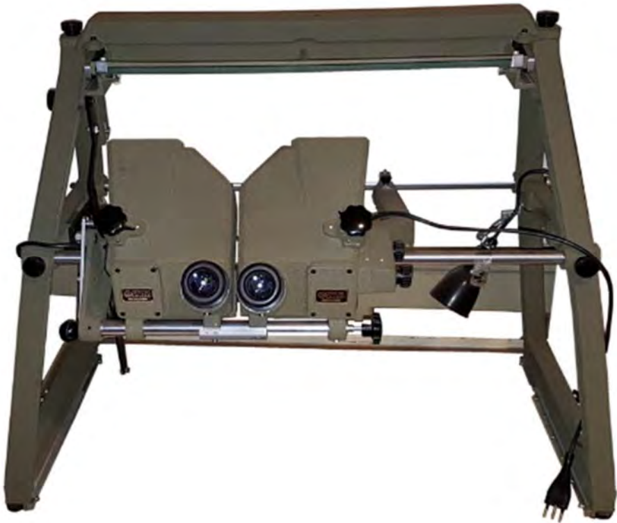
Stereovisor for photogrammetry. Officine Galileo. Circa 1960.
