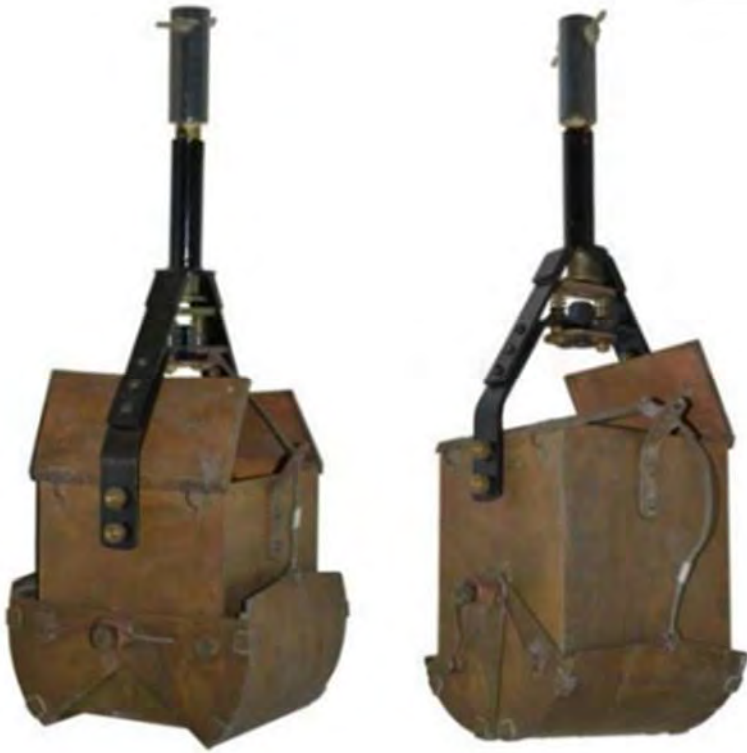
Ekman type dredge. Open (left) and closed (right). 1930s.
