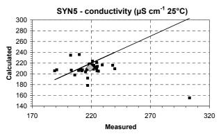
Fig 7.1 Comparison between the measured and calculated conductivity.
